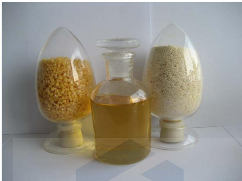
Titanate TCA-L12 with its powder masterbatch DLC-L12 and its pellet masterbatch MB-L12.
